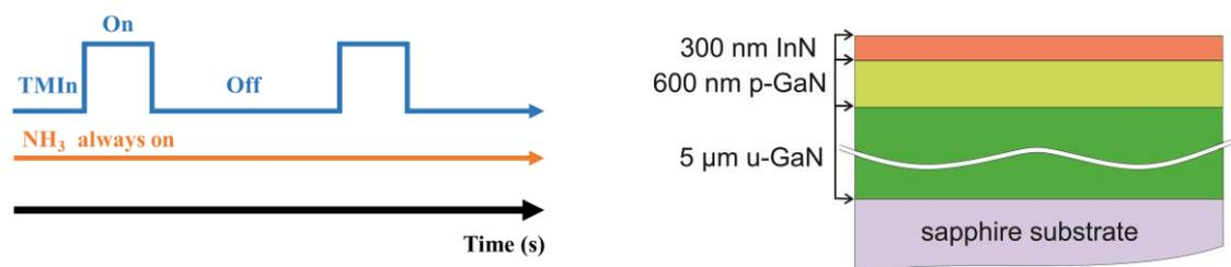
Figure 1. InN growth process (left) and final heterostructure (right).
