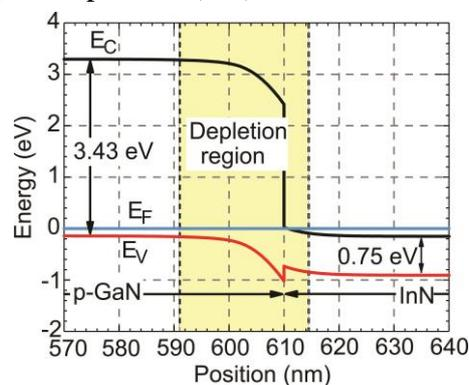
Figure 2. InN/p-GaN interface energy band diagram. The  $E_C$  stands for conduction band,  $E_V$  for valence band and  $E_F$  for Fermi level, respectively.
